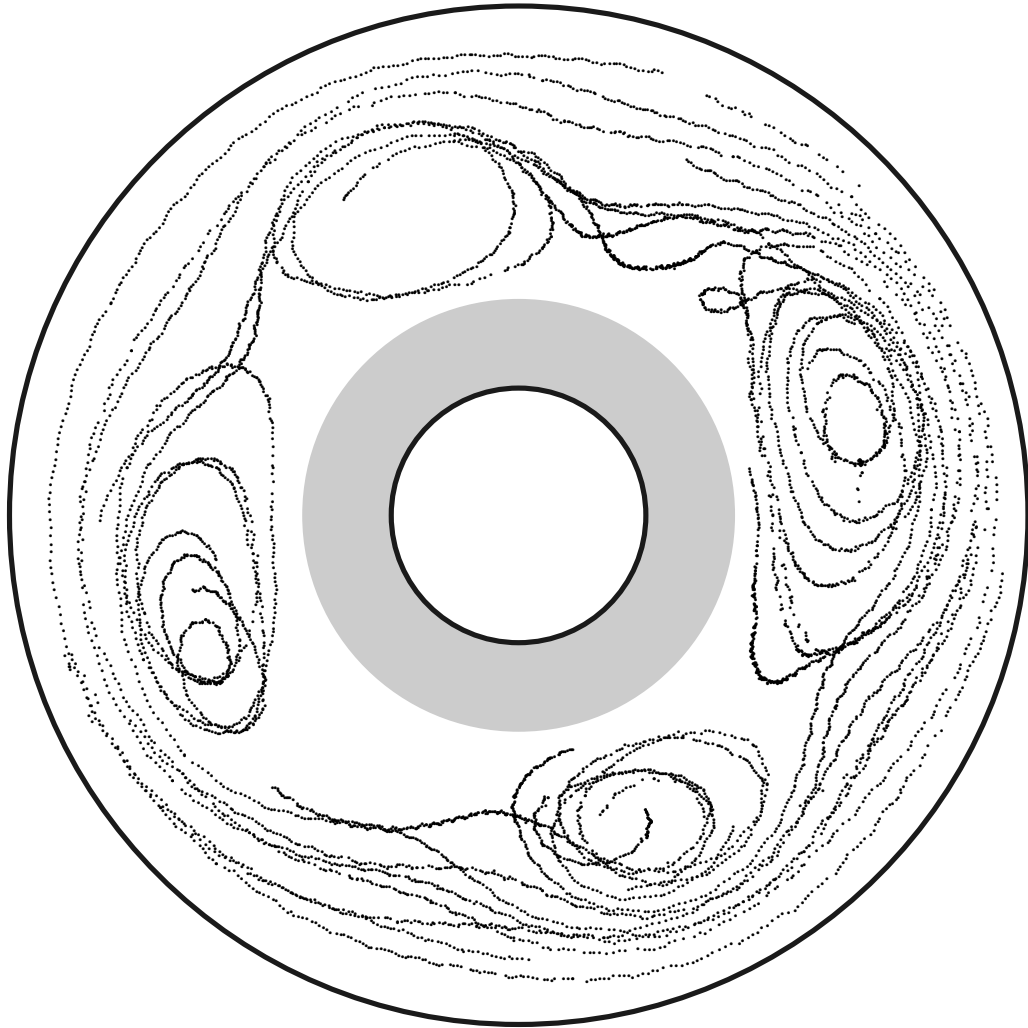
Figure 2: Streaks formed by 100s trajectories of 12 particles reveal four vortices. Weeks et al. show that the motion of these coherent vortices is chaotic. That is, a velocity spectrum, obtained by measuring velocity with a hot film probe, is broad band. Figure courtesy of Eric Weeks.
